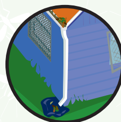
Clear debris that may block water flow in rain gutters.
